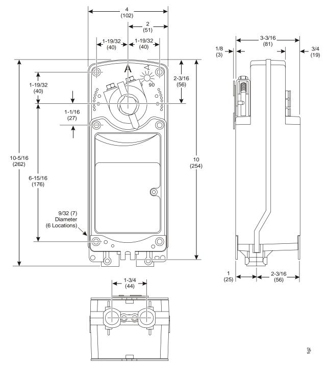
M9210-Bxx-3 Series On/Off Electric Spring Return Actuator Dimensions, in. (mm)
